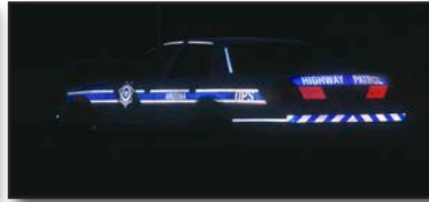
Figures 4.23a through 4.23c – Contour markings on police vehicles.
