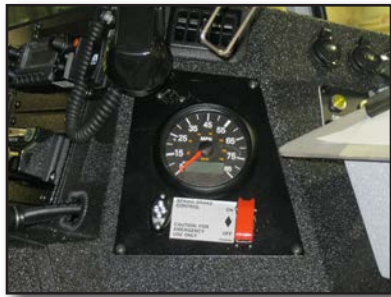
Figure 5.12 — Fire apparatus are equipped with speedometers on the officer's side of the vehicle. (Photo/Mike Wieder)
