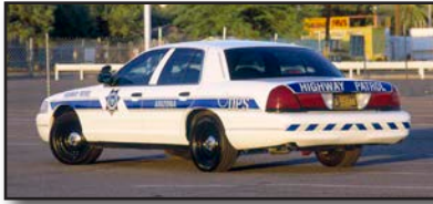
Figures 4.23a through 4.23c – Contour markings on police vehicles.
